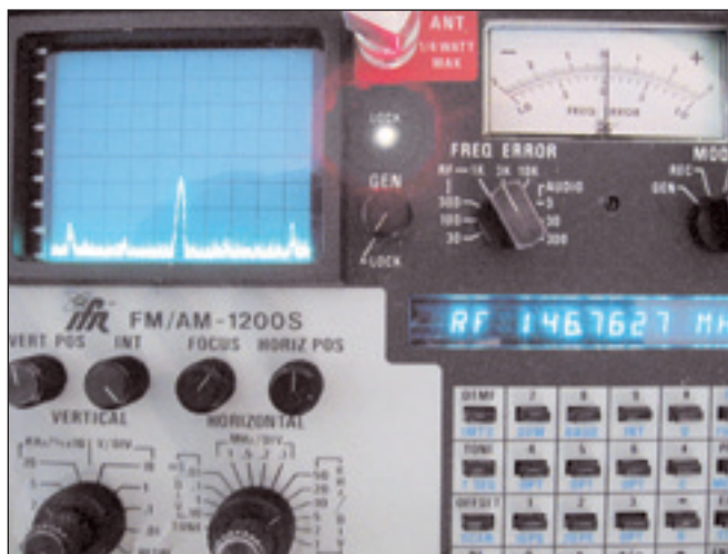
Figure 1 — The offending signal at 146.7627 MHz 30 dB above the noise.
